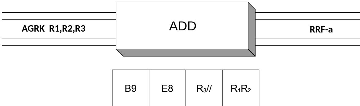
**ADD (AGRK)** is used to add two 64-bit signed, 2's complement, binary fields stored in grande registers, and produces a signed 64-bit sum that is stored in a grande register. Specifically, the second operand, R<sub>2</sub>, is added to the third operand R<sub>3</sub>. And the result stored in the first operand, R<sub>1</sub>. The second and third operands are unchanged by this operation.
