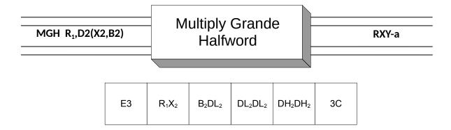
**MGH** (Multiply Grande Halfword) computes the product of a signed-binary halfword in memory (operand 2) with a signed-binary doubleword in the bits 0-63 of the general register R1. The 64-bit product is a signed binary integer and is placed in bits 0-63 of R1.
