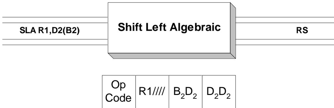
**SLA** is used to shift the 32 bits in the register specified by Operand 1 to the left. The number of bits that are shifted is indicated by Operand 2. The second operand address is **not** used to address data; instead, the base/displacement address is computed and the rightmost 6 bits are treated as a binary integer which represents the number of bits to be shifted. We will call this value the “shift factor”. This leads to two distinct ways of coding the shift factor:
