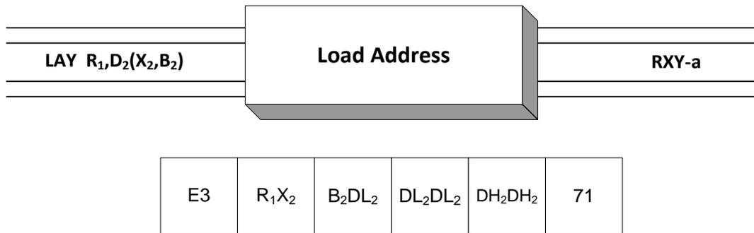
**LAY** is used to initialize the register specified by operand 1 with the address designated by operand 2. The number of bits that are loaded can be 24, 31, or 64 depending on the addressing mode. Operand 2 may be expressed using explicit notation or symbolic notation, or a combination of both. Remember that each byte in memory is numbered and that the number assigned to a byte is its address. The address of a field is the address of the first byte of the field. Consider the following example,
