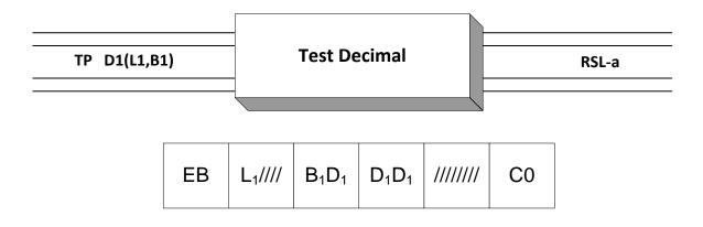
**TP** is an RSL-a instruction that is used to test a field to see if it is in a packed decimal format. A field of length 16 or less is in a packed decimal format if each byte contains two hex digits in the range 0-9, except the rightmost byte which contains a hex digit (0-9) followed by valid sign (hex values A, B,C, D, E, or F). The hex signs A, C, E, and F are positive, while hex signs B and D are negative.
